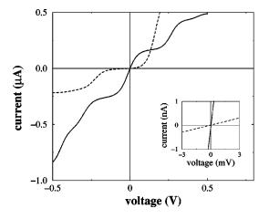
FIG. 6. Calculated *I*-*V* characteristics of the supported DB line, connecting two Au film pads 27 Å apart (six dimers). The solid (dashed) curve shows the *I*-*V* characteristic of the nondistorted (Peierls-distorted) DB line. The inset is a zoom around the origin.
