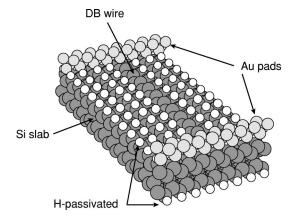
FIG. 1. Model of the metal-atomic wire-metal junction (defect) used in the ESQC calculation of the conductance of a wire consisting of 11 dangling bonds on depassivated silicon surface atoms. The dark gray spheres represent silicon atoms, while the light gray ones show the gold atoms of the contact pads. Both sides of the slab are saturated with hydrogen (white spheres), except along the defect line.
