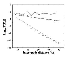
FIG. 4. Variation of the decimal logarithm of the transmission coefficient at the Fermi level as a function of the distance between the two pads, in the case of the perfect  $Si(001)-(2\times1)-H$  substrate (triangles), of the undistorted DB wire (circles), and of the Peierls-distorted DB wire (squares). The solid lines are linear fits. Note that there is no significant decrease for the metallic undistorted DB wire, although the net transmissivity is much smaller than one.
