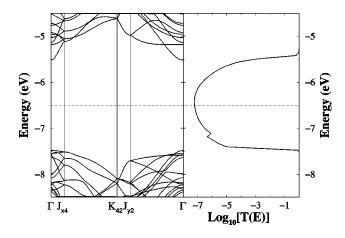
FIG. 2. Left panel: Calculated energy band structure of the slab representing the Si(001)-(2×1)-*H* substrate along the symmetry axis of the Brillouin zone corresponding to our 4×2 computational cell, following the notation of Watanabe *et al.* (Ref. 21). Right panel: Calculated decimal logarithm of the transmission coefficient between two Au film pads separated by 27 Å (six Si dimers) as a function of energy. The dashed line shows the position of the Fermi energy.
