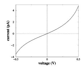
FIG. 3. Calculated current-voltage (I-V) characteristic of the Si(001)- $(2\times 1)$ -H substrate between Au film pads separated by 27 Å (six dimers).
